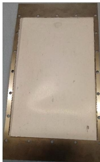
Figure 4 Gas diffusion electrode (gas side)
