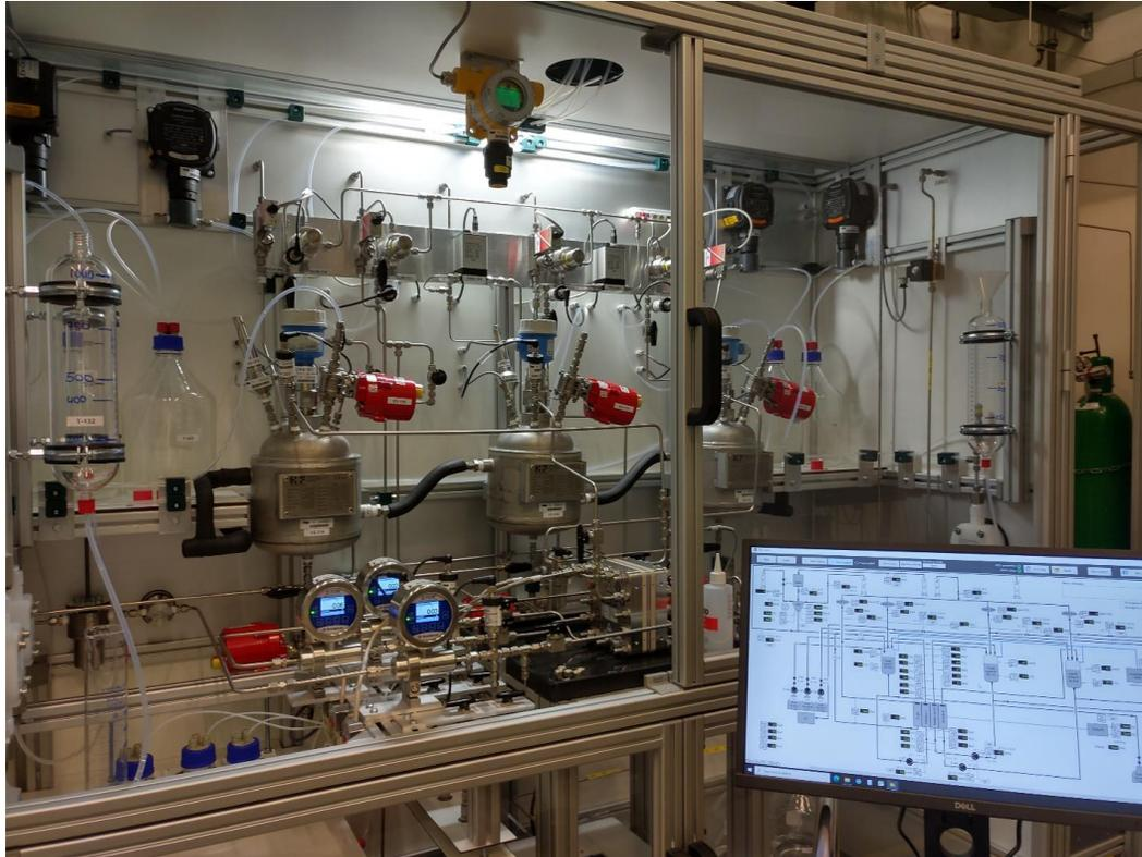
Figure 10. ELEKTRA – bench-scale demonstrator set-up and automation software
