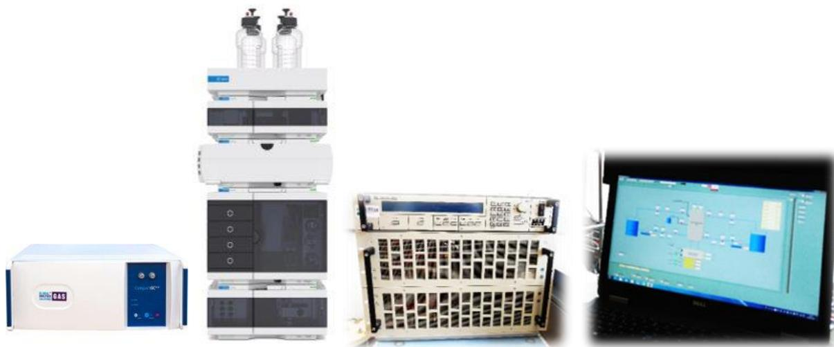
Figure 5. Peripherals of the bench scale feasibility system, from left to right, GC gas analyzer, HPLC, liquid sample analyzer, high power power supply and online process control and monitoring system.
