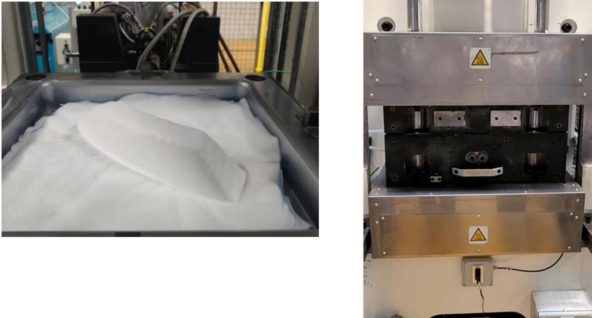
Figure 3: Manufacturing steps: Preforming of flax/PLA non-woven fabrics (left); Partial closing of mould at room temperature (right)
