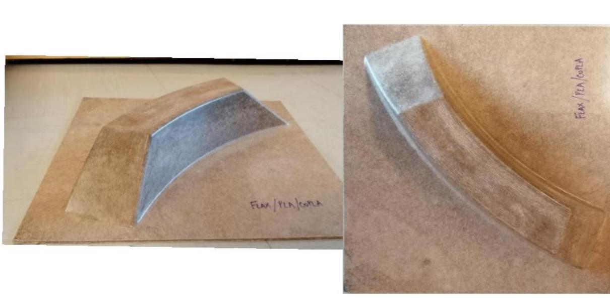
Figure 5: Flax/PLA/coPLA composite demonstrator
