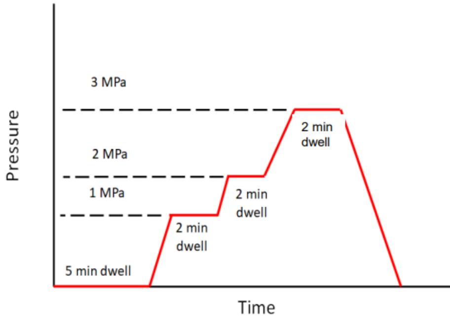
Figure 4: Consolidation cycle for Flax/PLA/coPLA composites
