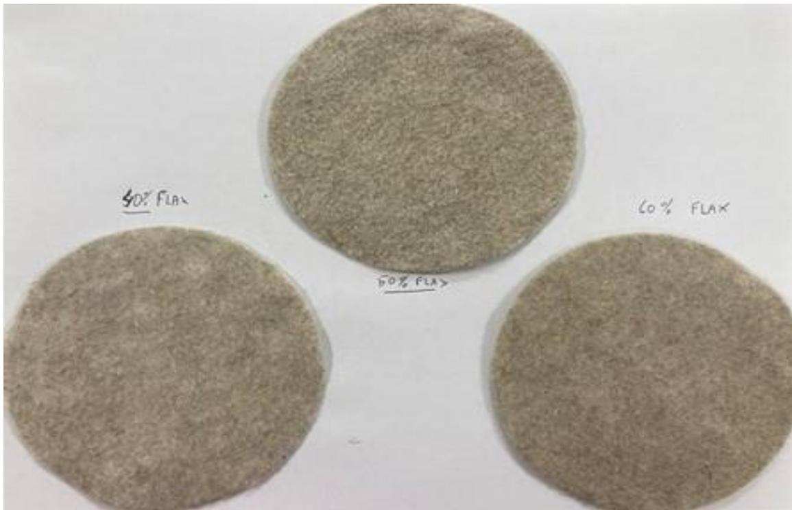
Figure 1: Samples of flax/PLA/coPLA fabrics
