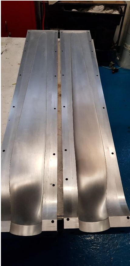
Figure 1 (left): Aluminium mould tool
