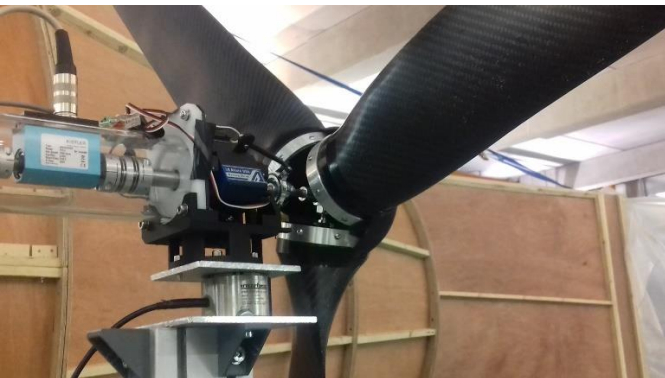
Figure 3: CFRP FLOW turbine blades installed in the University of Plymouth COAST Laboratory
