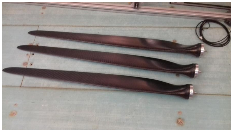
Figure 2 (right): CFRP FLOW turbine blades
