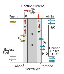
Figure 1 Schematics of hydrogen fuel cell
