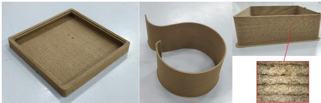
Figure 9: 3D printed demonstrators including detailed imaged indicated layer to layer bonding
