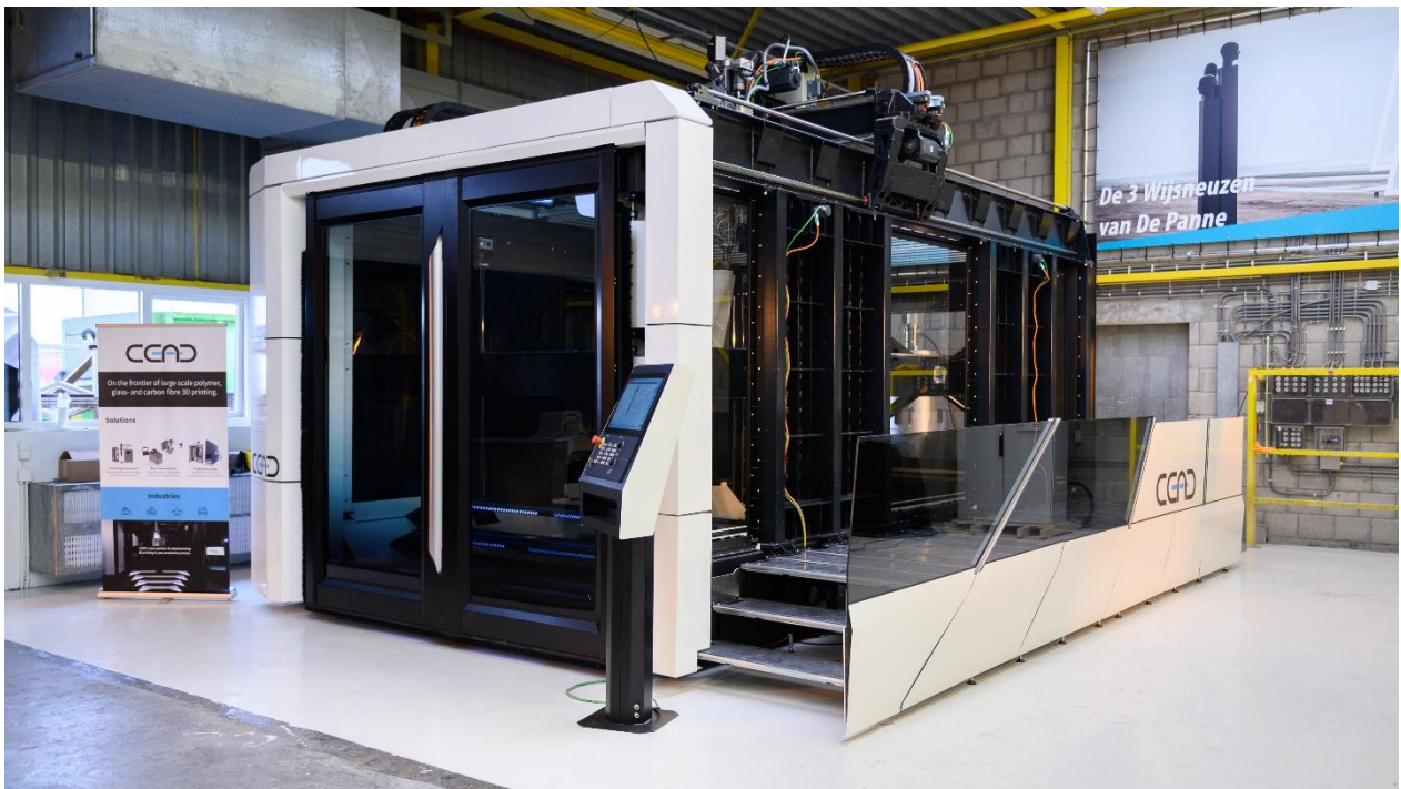
Figure 2: FDM-printer of Poly Products
