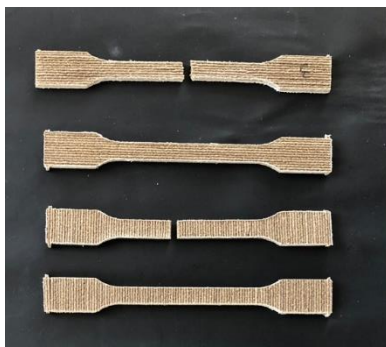
Figure 11: Representative dog bone specimens of the provided 3D printing materials/composites manufactured at 0° and 90°.
