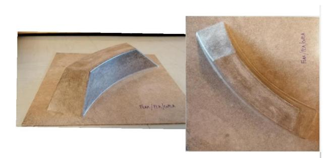
Figure 5: Flax/PLA/coPLA composite demonstrator
