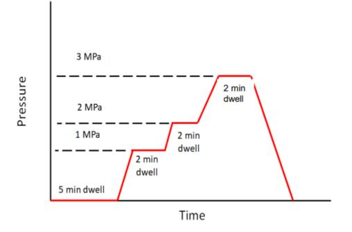
Figure 4: Consolidation cycle for Flax/PLA/coPLA composites
