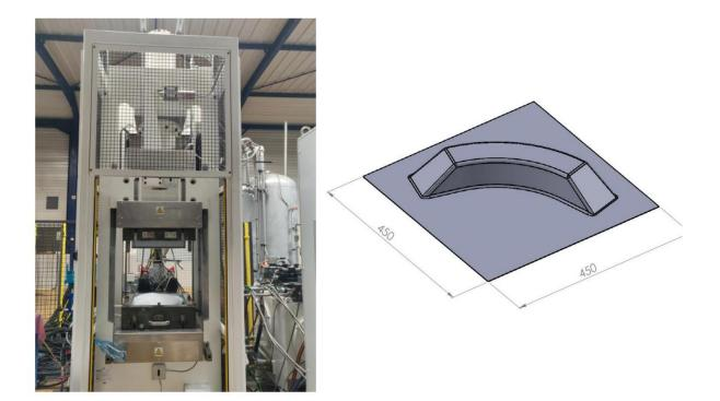
Figure 2: Hydraulic press used for compression moulding (left); CAD image of mold geometry and dimensions (right)
