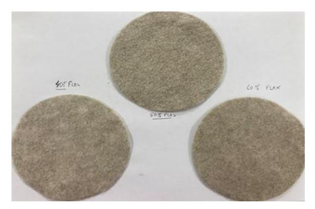
Figure 1: Samples of flax/PLA/coPLA fabrics
