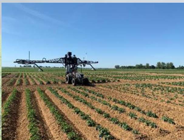
INNO-VEG project partner Arvalis measuring crop reflectance from potatoes using a vehicle mounted hyperspectral sensor
