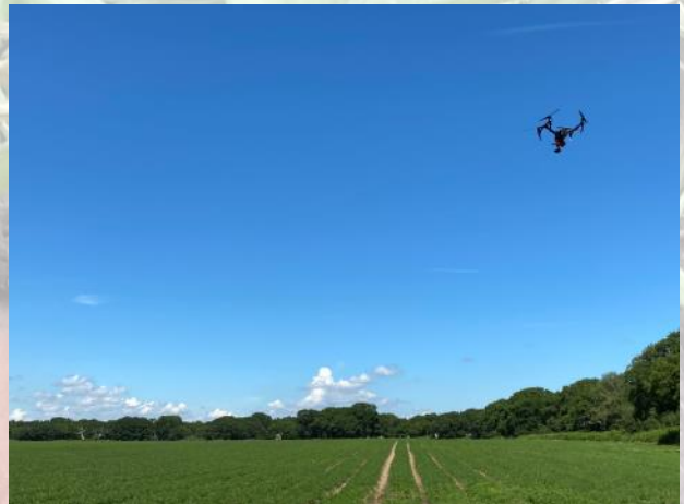
Collecting crop reflectance data from carrots using a drone mounted sensor.
