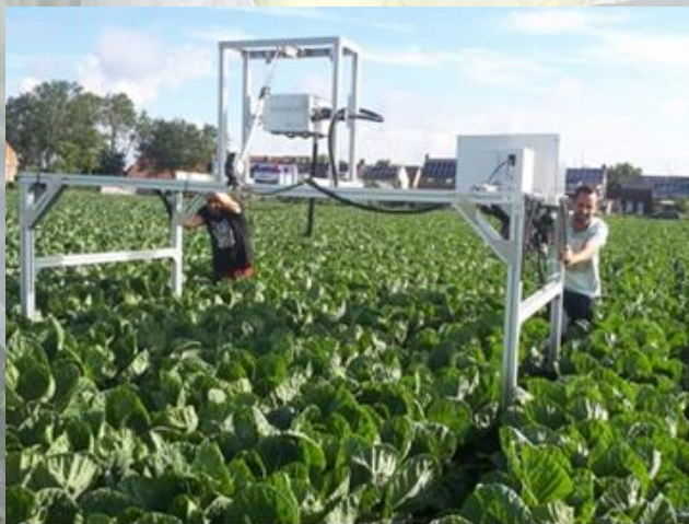
INNO-VEG project partner Delphy measuring crop reflectance from Brussels sprouts using a frame mounted multispectral sensor
