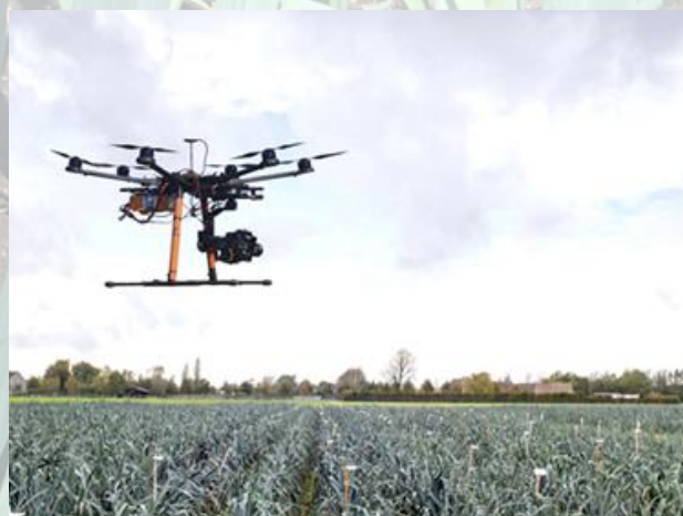
Collecting crop reflectance data from leeks using a drone mounted sensor
