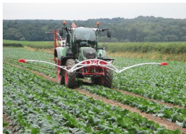
Figure 4. The Fritzmeier ISARIA multispectral sensor is mounted on the front of the tractor
