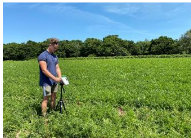
Figure 3. The handheld FieldSpec spectroradiometer has a field of view equal to half the measurement height; at a 1 m measurement height the sensor measures from a circular area 50 cm diameter
