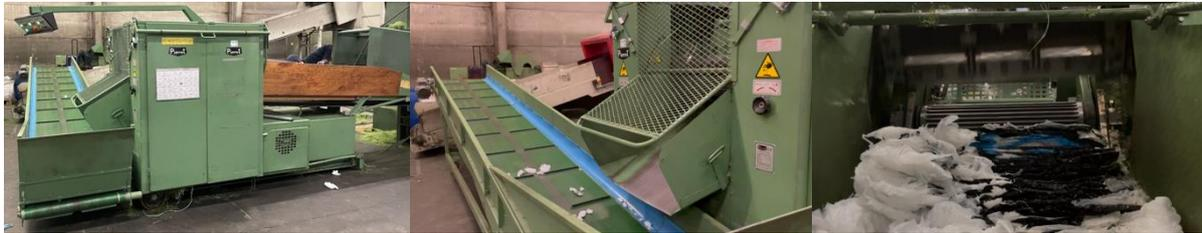
We were able to purchase this machine second-hand at a textile recycling company. It is ideal for reducing light materials in size. When handling films, especially post-packaging, it is very important not to shred the material but to keep it compact for the sake of the subsequent treatments. The waste we used in the picture above is comparable to the bags we expect to receive from the cities and as you can see the material remains dense.
