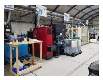
The wastewater treated by electrocoagulation then goes through a pre-filter for protection and then to the nanofiltration pilot system, which consists of two stages (first stage 2 membrane modules, second stage 1 membrane module). New phosphate recovery techniques will be tested on the nanofiltration concentrate, initially on a laboratory scale. The permeate of the nanofiltration pilot system passes through a softener, where calcium
