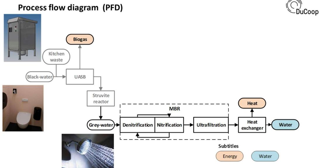
**Figure 1.** Process flow diagram of the DuCoop installation. Kitchen waste and black water are collected separately with a vacuum sewers system, after which they are pretreated with a biogas reactor (UASB) and struvite reactor. Further on, this stream is post treated together with the grey water.
