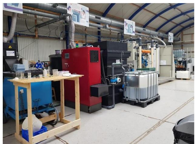
The wastewater treated by electrocoagulation then goes through a pre-filter for protection and then to the nanofiltration pilot system, which consists of two stages (first stage 2 membrane modules, second stage 1 membrane module). New phosphate recovery techniques will be tested on the nanofiltration concentrate, initially on a laboratory scale. The permeate of the nanofiltration pilot system passes through a softener, where calcium
