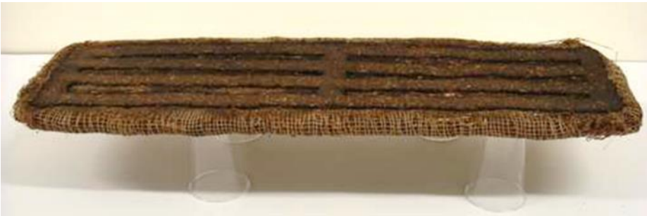
Figure3: Developed prototype of grass-stuffed geotextile roof or floor tile by HoGent
