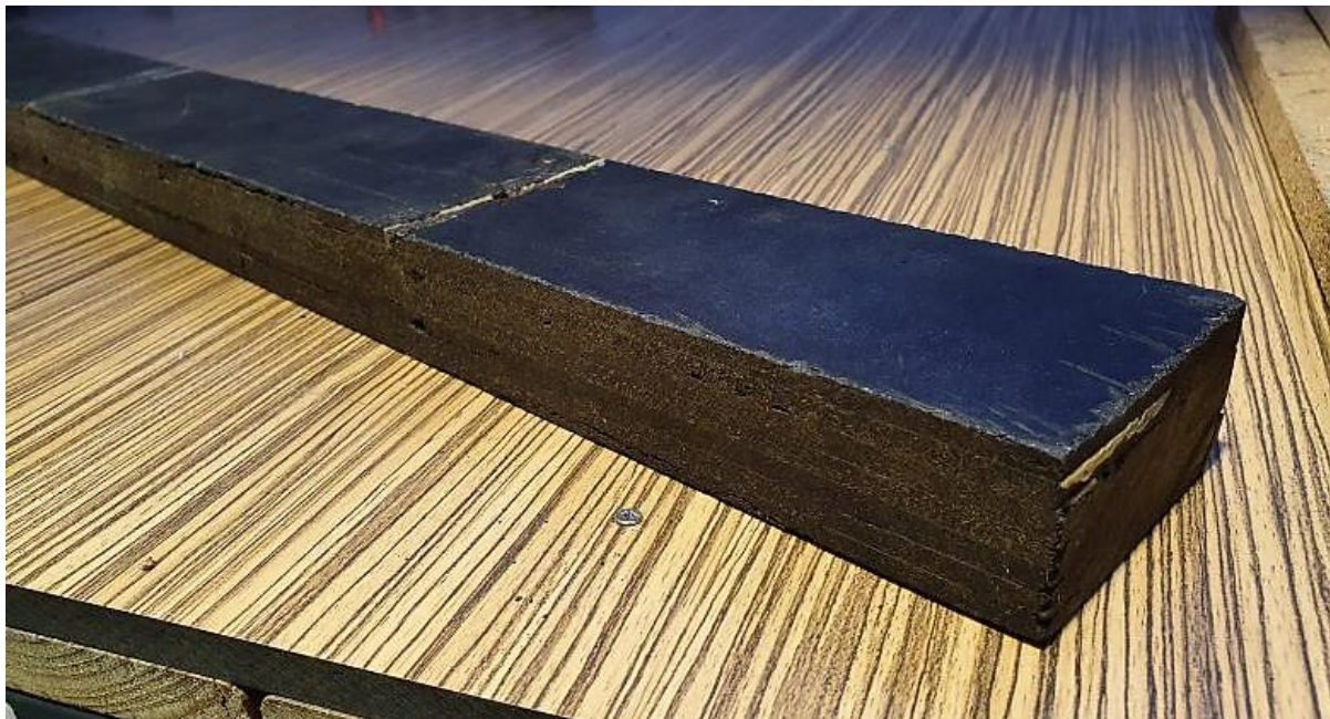
Figure 21: Developed prototype of a jetty board plank by Avans
